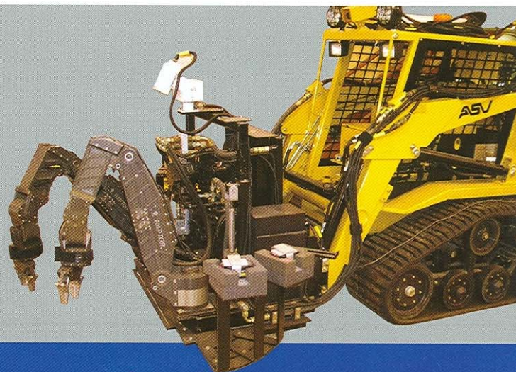
US Air Force "ARTS" vehicle, equipped with dual Raptor force feedback manipulator arms for the remote handling of unexploded ordnance.
